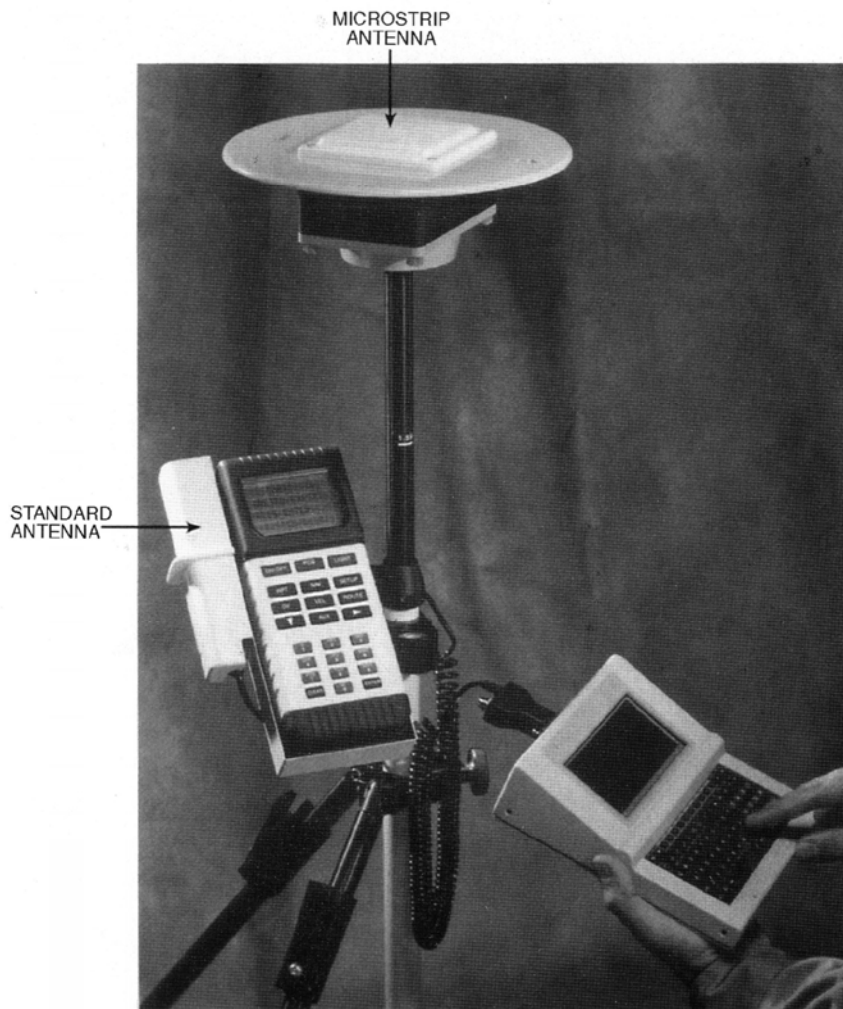
Fig. 20 Magellan 5-channel GPS NavPro 5000 GPS receiver shown with multipath resistant microstrip antenna and data collector
