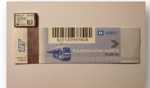
24 pin LCC (Leadless Chip Carrier): 12.2 x 16.0 x 2.4 mm, 1.6 g
